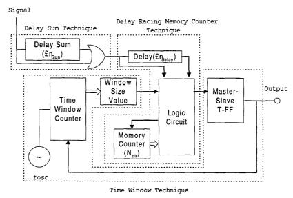
Fig.2 The Block Diagram for the Time Window, the Delay Racing Memory Counter, and the Delay Sum Techniques.
